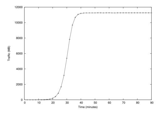
Figure 17: Traffic usage of an example worm
