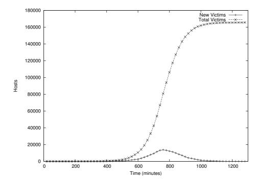
Figure 8: Sequential-scanning worm
